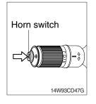
This switch is at the end of left side multifunction switch. On pressing, the horn sounds.
