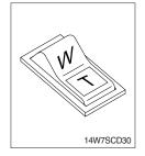
(1) This switch is used to select mode between travel and work.
