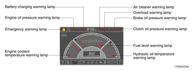
\* Each warning lamp on the top of the LCD pops up on the center of LCD and the buzzer sounds when the each warning is happened. The pop-up warning lamp moves to the original position and blinks when the select switch is pushed. And the buzzer stops. Refer to page 3-10 for the select switch.
