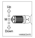
$\ensuremath{\textcircled{}}$  This switch is used to turn the head lights direction.
