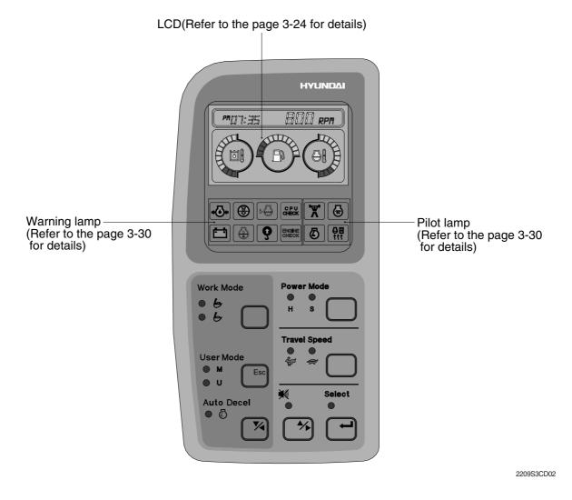
\* The warning lamp lights ON and the buzzer sounds when the machine has a problem. In this case, press the buzzer stop switch and buzzer stop, but the warning lamp lights until the problem is cleared.
